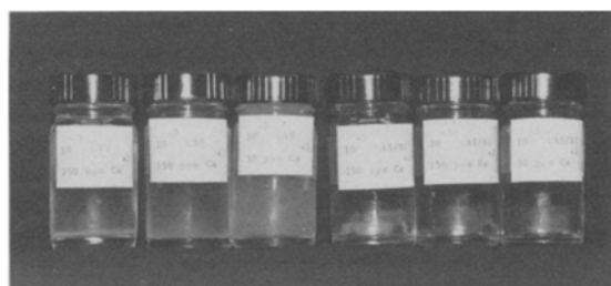
FIG. 2. From left to right, solutions of LAS at 250 ppm, 150 ppm and 50 ppm hardness and LAS/Alfonic® 1214-60 alcohol ethoxylate at 250 ppm, 150 ppm and 50 ppm hardness.
